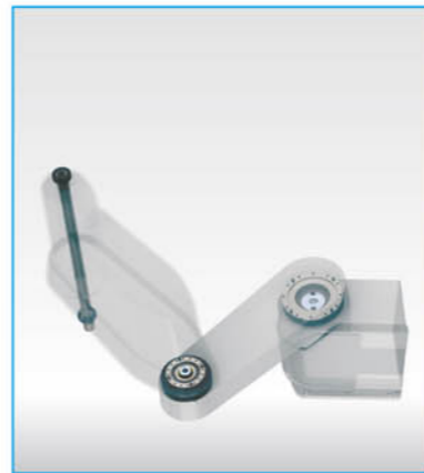
Selective Compliance Assembly Robot Arm
